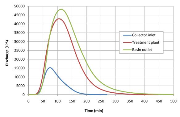
Figure 5. Hydrographs for each outlet in post-collector model
