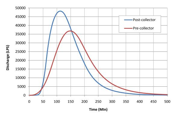
Figure 4. Total outflow hydrographs for pre- and post collector models.
