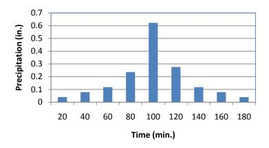
Figure 1. Incremental distribution of the 3-hour design storm.
